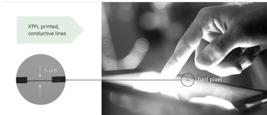
Figure 3 Removing local defects in conductive structure is needed in most cases as conductive electrodes are used in semi-finished products whose production cost is a significant part (even 50%–70%) of the cost of the final product. The XTPL solution ensures precise, fast and effective open defect repair, significantly increasing the efficiency of advanced production lines.
